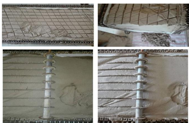
Fig. 8 Photographs of racking patterns of the PG cake while moving over the rotation belt
