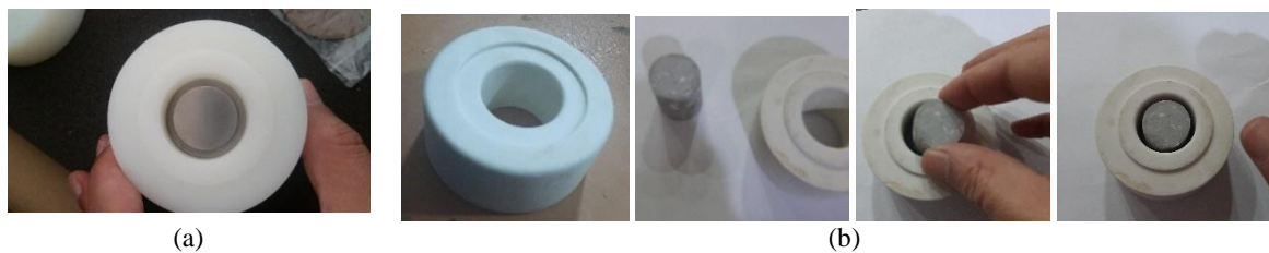
Fig. 7 Samples insertion in the holder that is attached in the measurement of thermal conductivity: (a) Shows the reference sample used for device calibration, (b) sample insertion into the measurement device.
