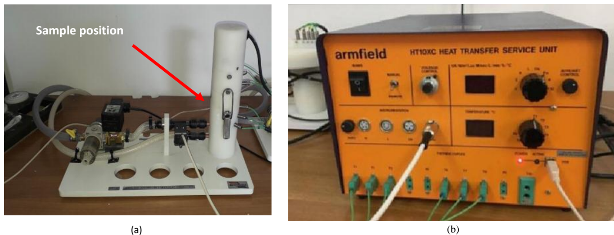
Fig. 8 (a) Armfield Linear Heat Conduction Accessory: Computer Controlled Linear Heat Conduction-HT11C unit, (b) Heat transfer service unit, HT10XC.
