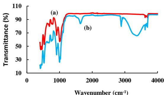
**Fig.2** FTIR spectra of (a) raw Kaolin and (b) modified Kaolin.
