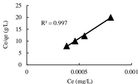
**Fig. 4** Langmuir isotherm at 60°C.
