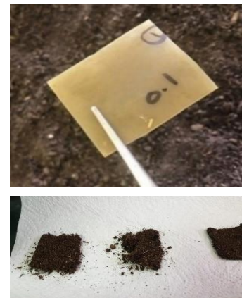
Fig 13. Biodegradability test (a) Kaolin sample before poured in soil. (b) Kaolin sample after two weeks
