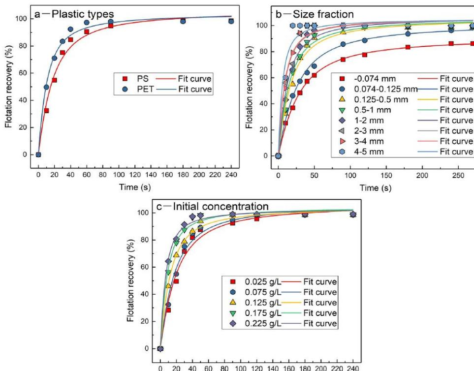
**Fig. 7.** The flotation removal of PS MPs with different plastic types (a), size fraction (b), and PS MPs initial concentration (c). Reprinted with permission from (Zhang *et al.* 2021).
