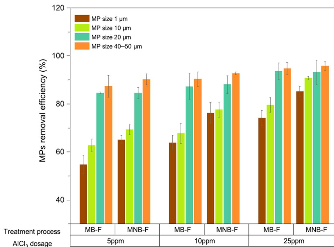
**Fig. 9.** The removal efficiency of MPs by microbubble flotation (MB-F) and combined microbubble with NBs flotation (MNB-F) showing comparison of the removal efficiency of MPs with different sizes (1–50  $\mu\text{m}$ ) and at different doses of coagulant by MB-F and MNB-F. Reprinted with permission from (Jia *et al.* 2024).
