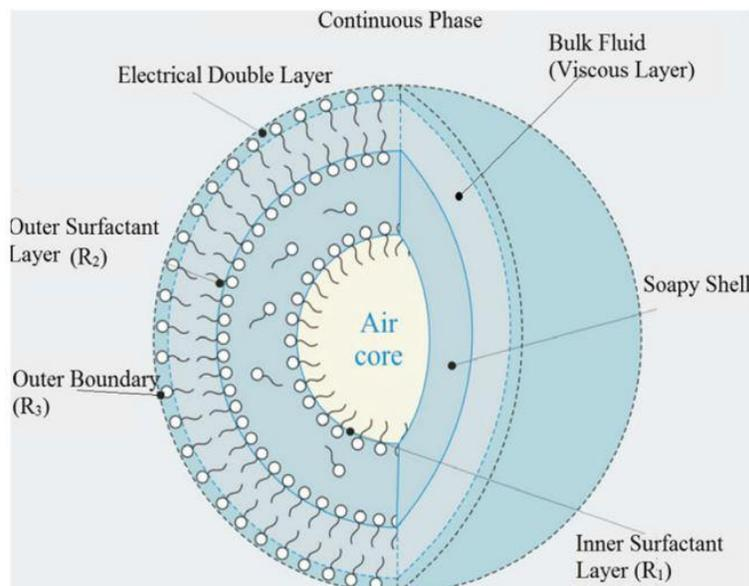
**Fig. 3.** Schematic of a colloidal gas apton (CGA). Reprinted with permission from (Sebba 1985).
