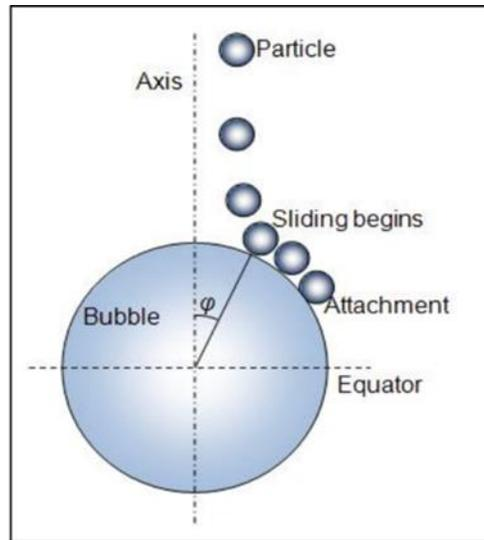
Fig. 4. A schematic representation of a particle sliding over a gas bubble surface. Reprinted with permission from (Verrelli *et al.* 2012).
