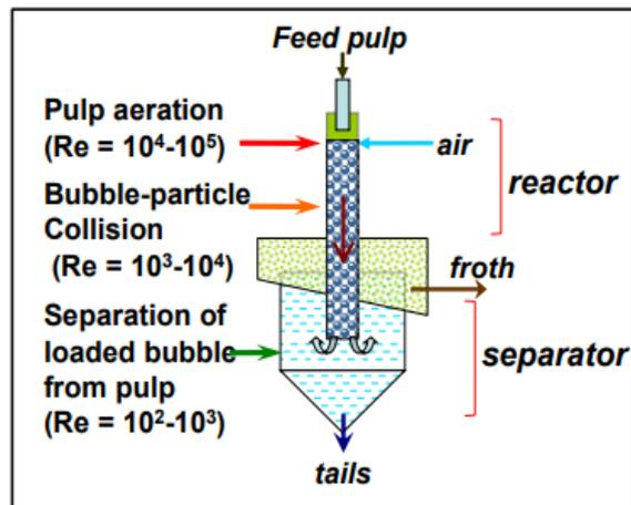
**Fig. 6.** A schematic diagram of a flotation cell of type reactor-separator. Re is the Reynolds number. Reprinted with permission from (Fornasiero and Filippov 2017).
