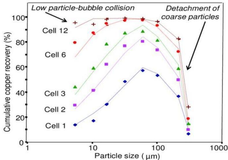
Fig. 5. A typical flotation recovery as a function of particle size. Reprinted with permission from (Ralston *et al.* 2007).
