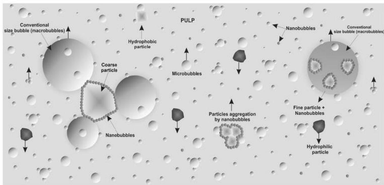
**Fig. 8.** A schematic representation of the mechanisms involved in the enhanced flotation using nanobubbles (NBs). Reprinted with permission from (Rosa *et al.* 2018).
