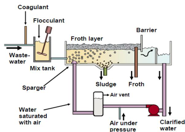
**Fig. 2.** A schematic diagram of a dissolved air flotation (DAF) unit. Reprinted with permission from (Hubbe *et al.* 2016).
