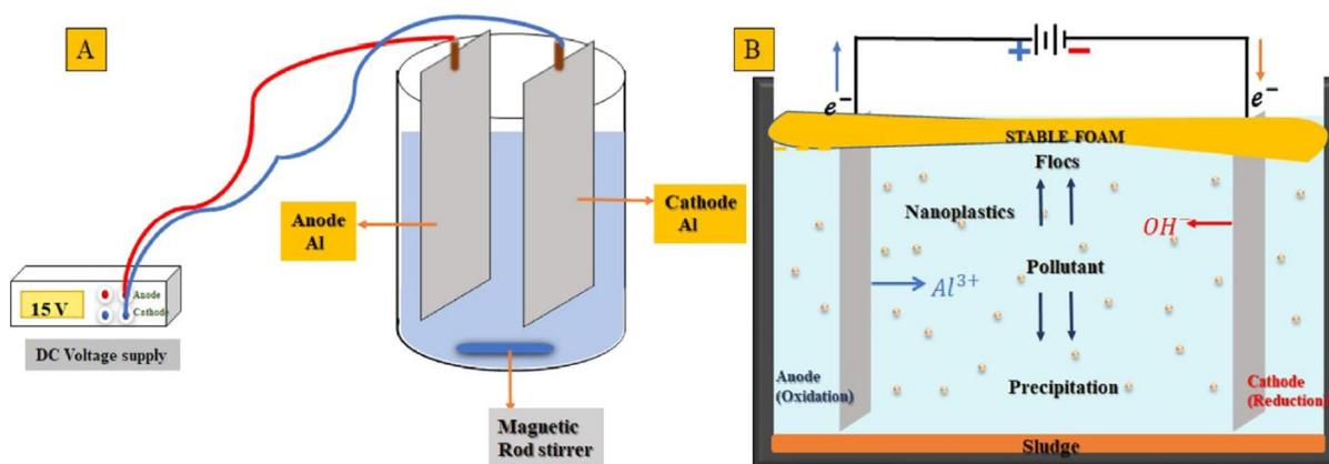
**Fig. 1.** Schematic diagram of an EF flotation unit: a) experimental setup, b) removal mechanism of NPs by the EF process. Reprinted with permission from (Pawak *et al.* 2023).
