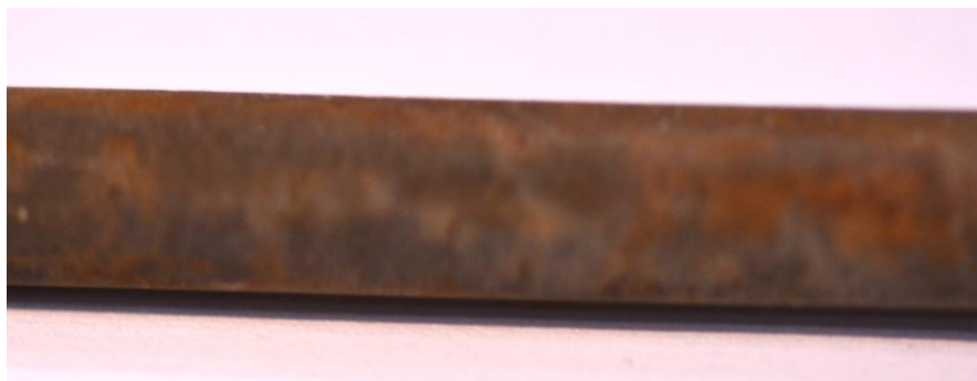
Fig. 2. Mild steel after immersion in 1 M of H 2 SO 4 only (48 hrs).
