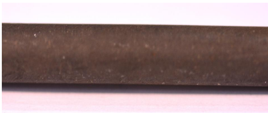
Fig. 3. Mild steel after immersion in 1 M of H 2 SO 4 with essential oil extract included (48 hrs).
